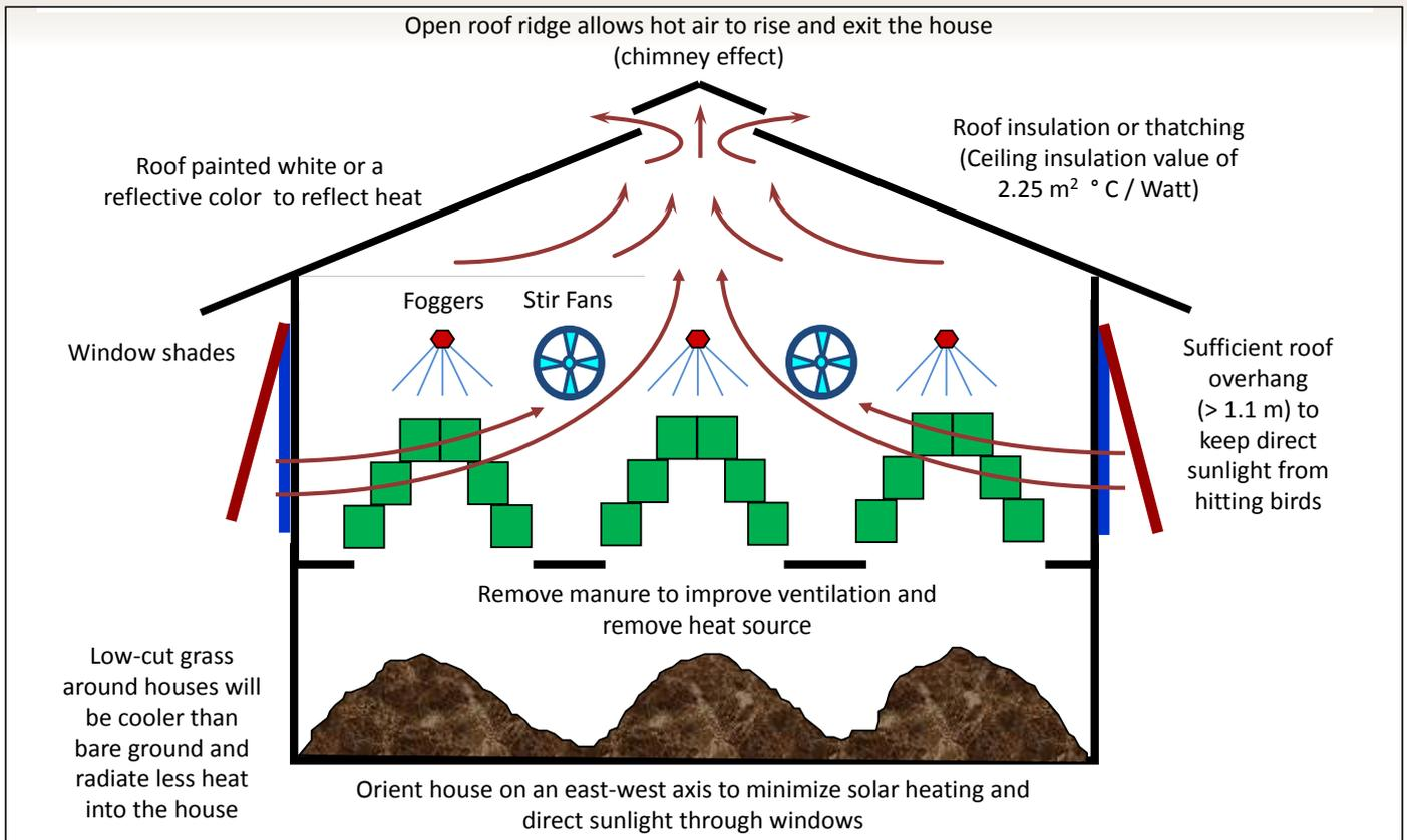
Figure 7. Open house design for reducing heat stress.
